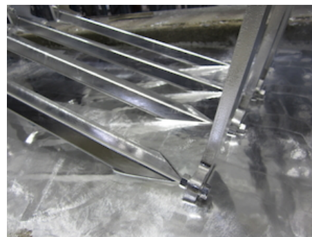
OAT104 - Standard finish GALVANISED for HTL frame
