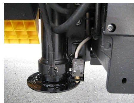
OAH013.40.300 - Hydr.stabilising leg straight 2T 300mm
