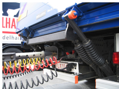
OAF001 - Lift arm for trailer coupling LMK
