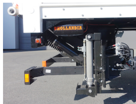
OAH011.LE - Articulated stabilising legs 10T on LSU>4T
