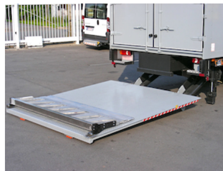
OAP404.1 - Reinforced foldable point (1x) on DHL*
