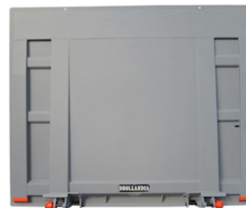
OAP304 - Steel platform flat between the main beams
