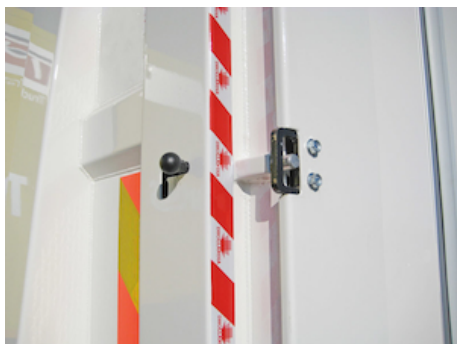
OAP422.R - Standard lock on STEEL platform R
