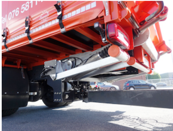
Bumper bar in elevated position for combi-ride with trailer
