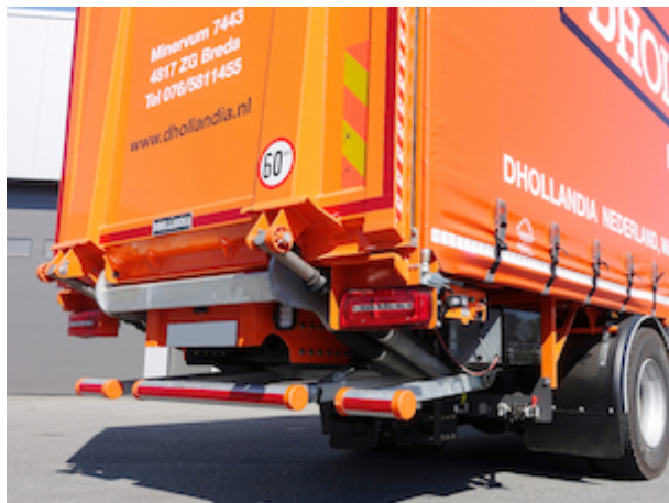
Bumper bar lowered to legal bumper height for a solo-drive without trailer
