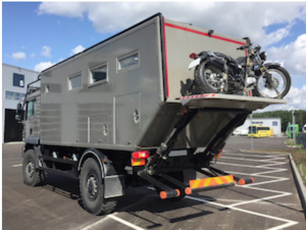
Tail lift used for military or civil off-road applications
