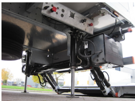
OAH013.60.LE - Hydr.stabilising leg straight 4T LE...mm
