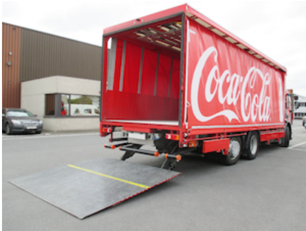
Tail lift used for regular distribution transport (e.g. supermarkets, drinks distribution)
