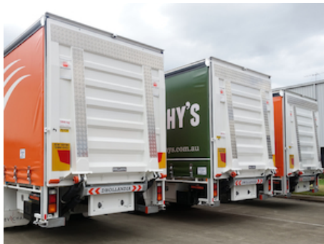
Long platforms available, forming the rear closure of the body aperture
