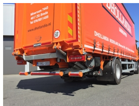
OAU004 - DH-LV for draw-bar coupling + fold-away bumper
