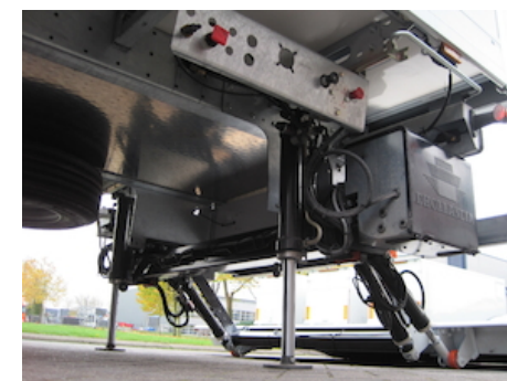
OAH013.60.LE - Hydr.stabilising leg straight 4T LE...mm
