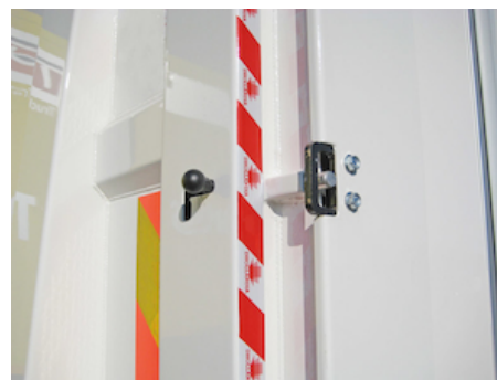
OAP422.R - Standard lock on STEEL platform R
