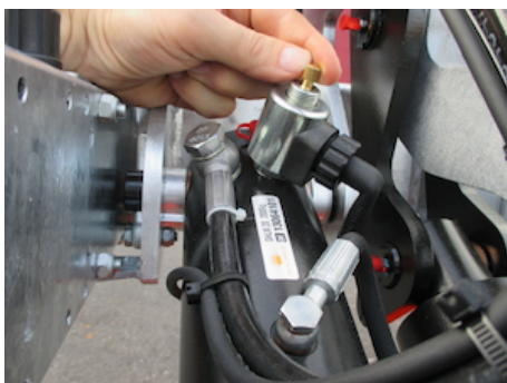
Manual emergency operation on all electrovalves
