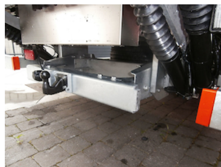
OAF103 - Preparation LM bumper for ball coupling
