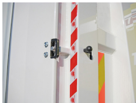
OAP422.L - Standard lock on STEEL platform L
