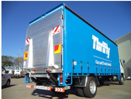
Weight-saving aluminium platform with anti-slip surface
