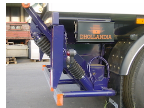
OAU005 - Dh-LMP/ESP execution for very short overhang
