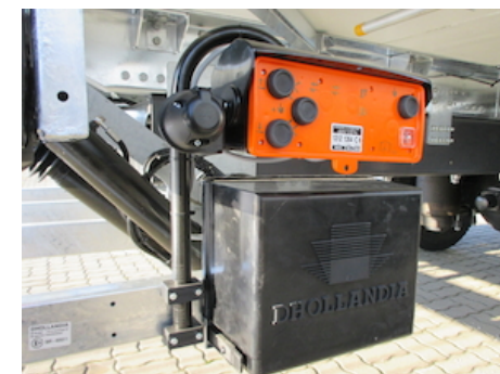
OAM025 - Adjust. support for control behind power pack
