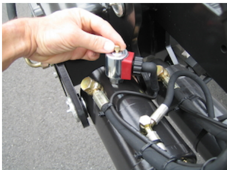
Manual emergency operation on all electrovalves
