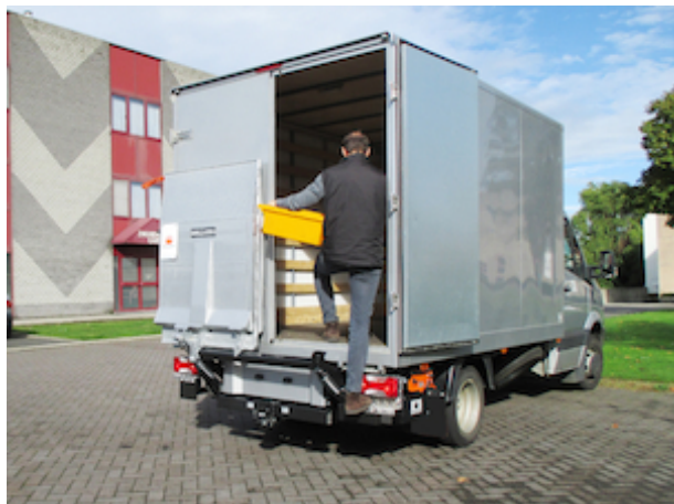
In closed position, the tail lift still offers free access to the loading space inside the body.
