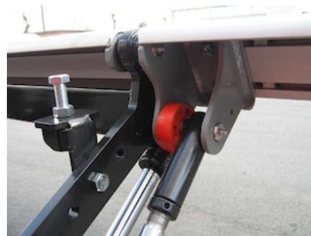
OAM006 - Stop for lift arm against underside of body
