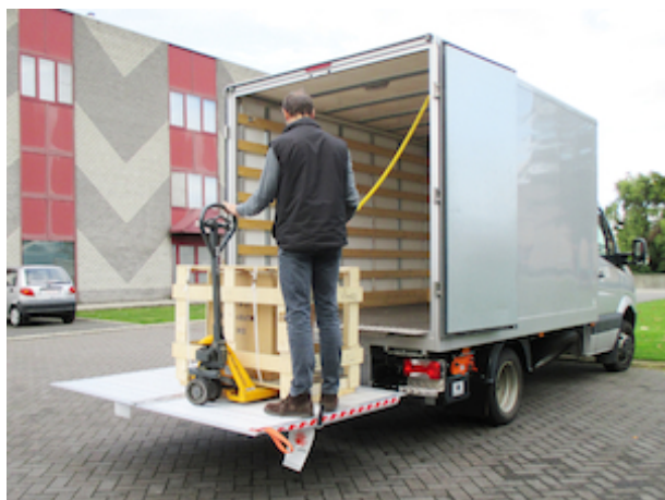
The foldable platform can be deployed into a full-width platform in a matter of seconds.
