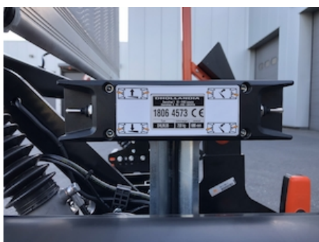
OAE048.0 - Control unit with 2 toggle-switches
