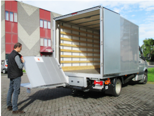
Half-width platform, or foldable platform [option OAP406] made of lightweight aluminium profiles
