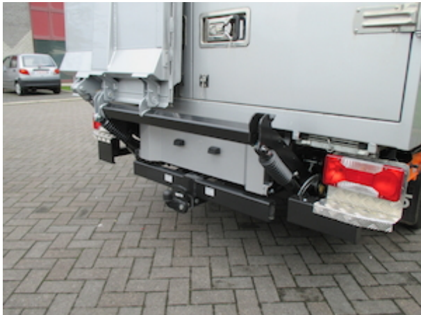
2 hydraulic lift cylinders and a wide arm with guarantee maximum platform stability
