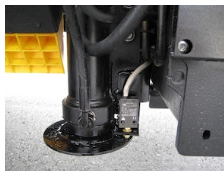
OAH013.40.300 - Hydr.stabilising leg straight 2T 300mm
